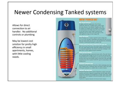
Heat+cool: Ducts provides distribution, can add ventilation, no DHW
