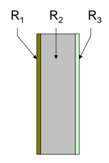
$R_{T} = R_{1} + R_{2} + R_{3}$
