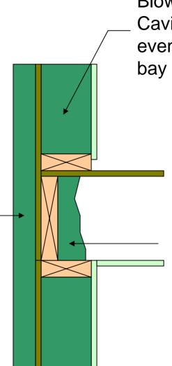
Blown/Sprayed Cavity insulation to evenly fill the stud bay
