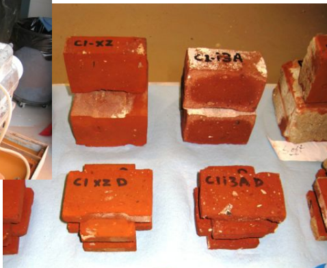
Multiple small slices from each of several different bricks
