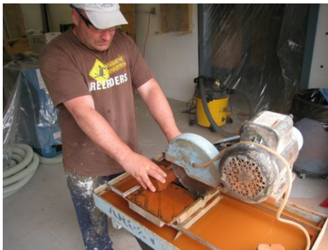
Multiple small slices from each of several different bricks
