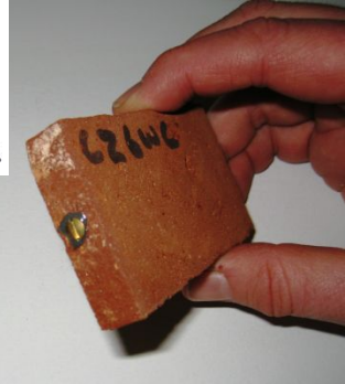
Figure 4-2 Typical brick sample with measuring pin targets.
