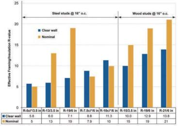
\* ci denotes a layer of continuous insulation with no framing penetrations
